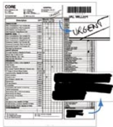
Conventional Scanning Without VRS: Scanning the same form in black-and-white (bitonal) makes the pencil text easier to read and reduces the file size to 88 Kbytes. But the highlighted text is completely lost, and the shaded boxes become shades of gray, which would confuse a system that is looking for the check marks.
